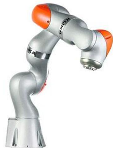
collaborative and sensitive LBR iiwa robot is available in two versions with payload capacities of 7 and 14 kilograms.
